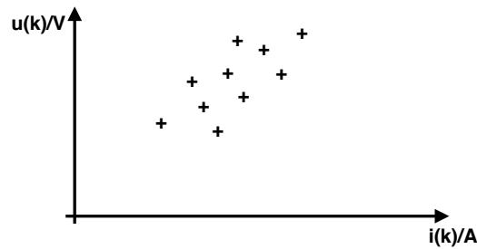
Figure 1.3: The same measurements in a voltage-current diagram.
