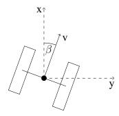
The system can be described by a state space model with three internal states. The state vector  $\mathbf{x} = [x \ y \ \beta]^{\top}$  contains the position of the robot in the X - Y plane and the deviation  $\beta$  from its initial orientation. The system can be controlled by the angular velocities of the wheels:  $\mathbf{u} = [\omega_L \ \omega_R]^{\top}$ . The output of the system is the position of the robot:  $\mathbf{y} = [x \ y]^{\top}$ . The model follows as
