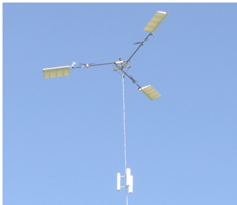
Figure: Real world rotorkite prototype, Copyright © 2019 Bladestips Energy
