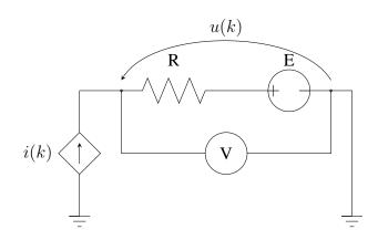
You obtain two datasets each containing N measurements of the voltage u(k) for different values of i(k). The first dataset contains  $\{u_1(k)\}_{k=1}^N$  and  $\{i_1(k)\}_{k=1}^N$  and the second dataset contains  $\{u_2(k)\}_{k=1}^N$  and  $\{i_2(k)\}_{k=1}^N$ . For cleaner and simpler notation, we omit the dataset indices, e.g. instead of  $u_1(k)$  and  $u_2(k)$  we write u(k) but mean both.
