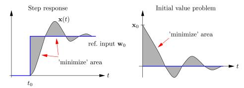
For a good controller performance, one would demand for a fast response and little overshooting, hence for minimizing the shaded areas. Meanwhile, one would also want to save the energy used by the controller in implementing control actions. The performance index for the LQR controller is introduced
