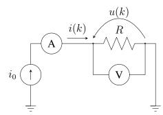
Imagine you are sitting in a class of 200 electrical engineering students and you want to estimate the value of R using Ohm's law. Since the value of the current  $i_0$  flowing through the resistor is not known exactly, an ammeter is used to measure the current i(k) and a voltmeter to measure u(k). Every student is taking 1000 measurements. The measurement number is represented by k. We assume that the measurements are noisy:
