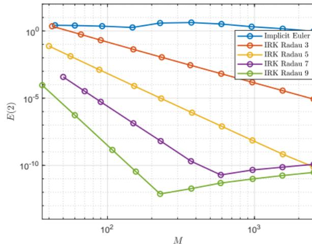
Integration error  $E(T)$  at time  $T = 2$  vs. total number  $M = s N$  of collocation points, for different Radau IIA methods.
