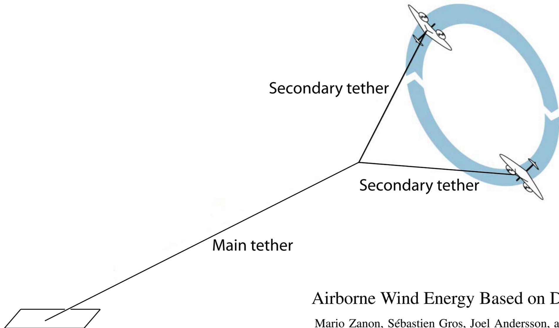
Airborne Wind Energy Based on Dual Airfoils
