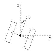
The system can be described by a state space model with three internal states. The state vector  $\mathbf{x} = [x, y, \beta]^{\top}$  contains the position of the robot in the X - Y plane and the deviation  $\beta$  from its initial orientation. The system can be controlled by the angular velocities of the wheels:  $\mathbf{u} = [\omega_{\mathrm{L}}, \omega_{\mathrm{R}}]^{\top}$ . The output of the system is the position of the robot:  $\mathbf{y} = [x, y]^{\top}$ . The model follows as
