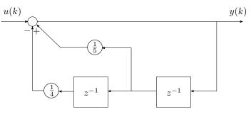
Figure 1: Diagram of a discrete time system
